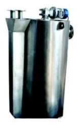
To get good performance from sludge dewatering machine the sludge has to be condition with suitable flocculent .it has been found that a slow agitated tank with a residence time of upto 2-3 minutes is normally sufficient to do a good job of flocculation .after the mixing of sludge and poly electrolyte strong large size flocks will be obtained which are fed to the dewatering machine.
