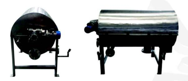
The internally feeding system is fine screen consist of a tank and a spiral connected to the drum for conveying of screening material. The screen is compose of perorated plate whole diameter is as big as the desired opening size. The drum is supported by suitable shaft and is operated by geared motor.
